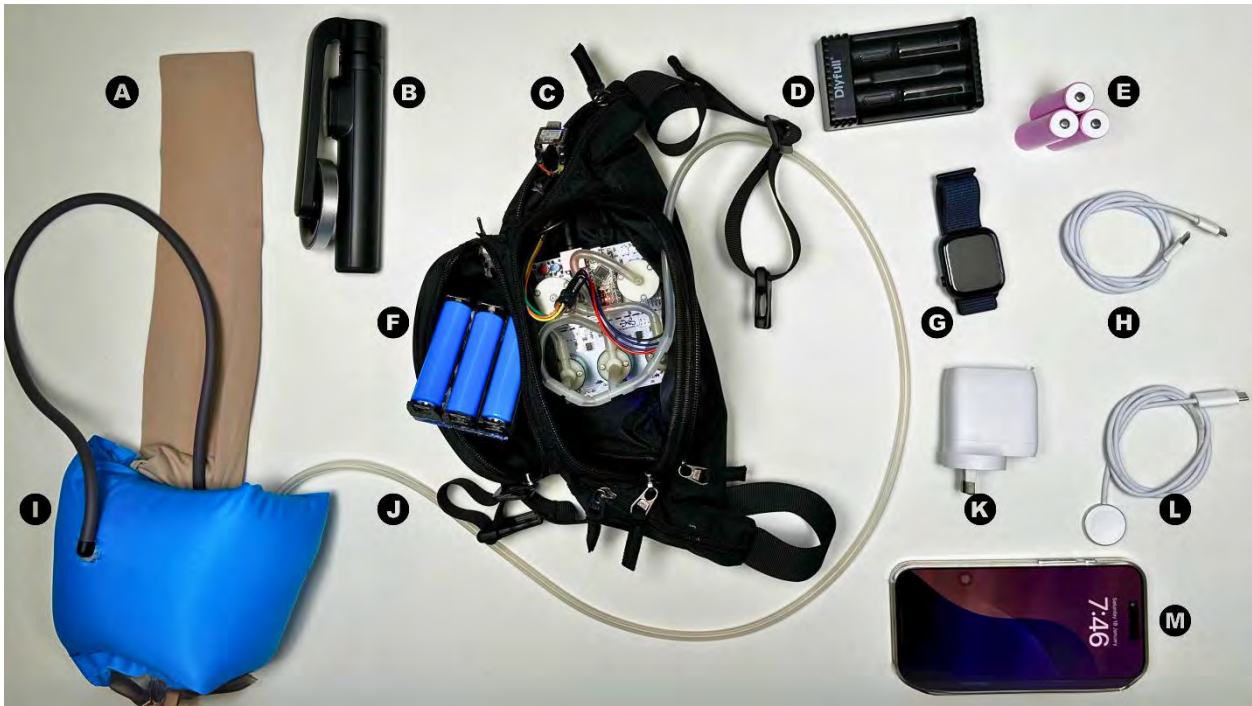
Figure 36: Study kit: A. The bodily extension with an air tube. B. Portable tripod for capturing study sessions (optional). C. Waist bag containing the pneumatic microcontroller and batteries. D. Battery charger. E. Spare rechargeable batteries. F. Pneumatic microcontroller setup with wiring and components. G. Smartwatch for physical activity tracking. H. Charging cable. I. Inflatable sleeve. J. Transparent air tube connecting the controller to the bodily extension. K. Power adapter for charging devices. L. Magnetic charger for the smartwatch. M. Mobile phone, used for recording the study experience (recording was optional for participants).
