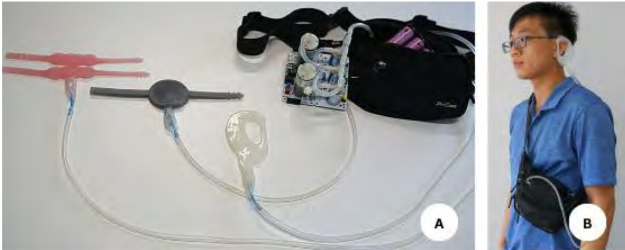
Figure 13: A) The pneumatic controller in a waist bag along with the three bodily extensions (from left to right: “Greetings”, “Take a break”, and “Pardon?”); and B) A person wearing the “Pardon?” bodily extensions.
