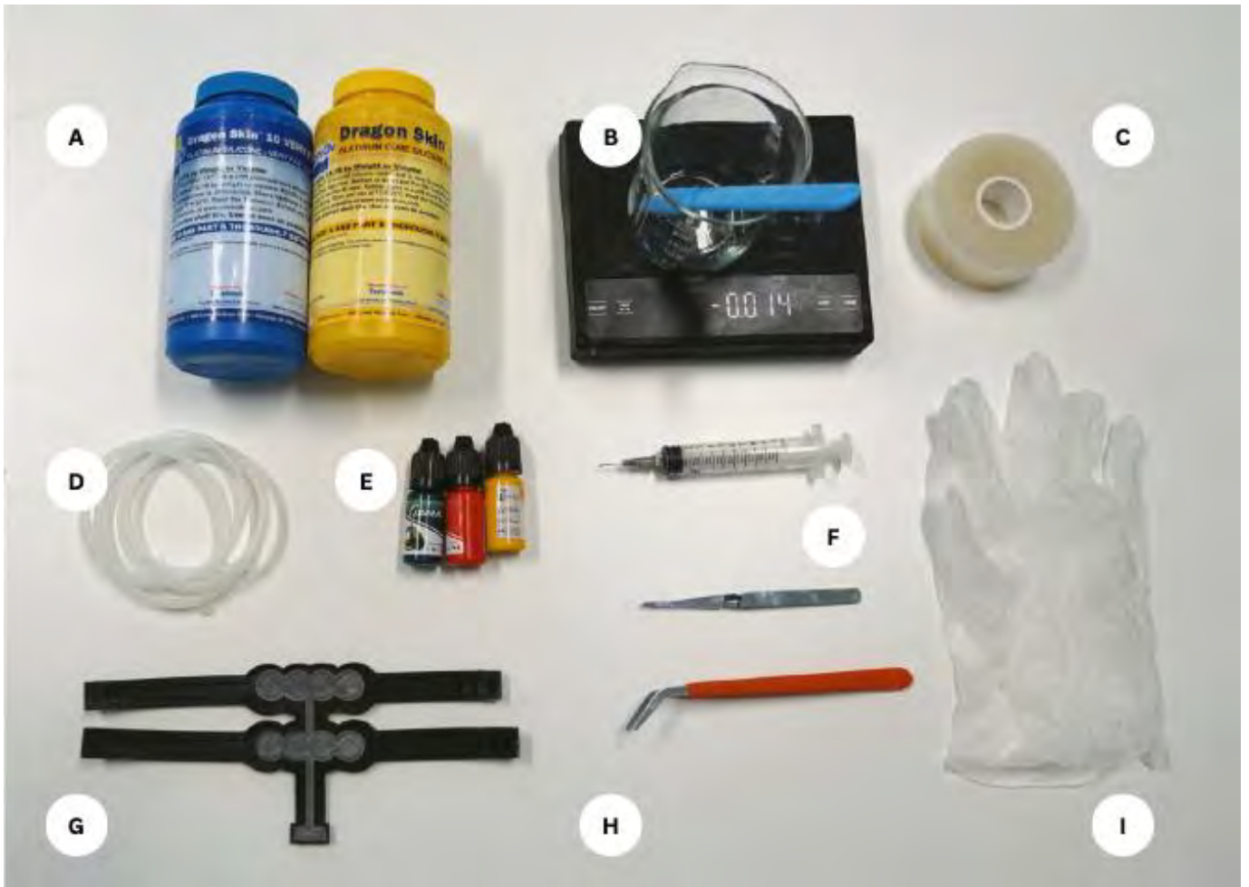
Figure 15: Fabrication kit for creating silicone-based bodily extensions. A) Liquid silicone; B) Weighing scale and a beaker for mixing silicone; C) Silicone tape for sealing the bodily extensions post fabrication; D) Silicone tube to connect the bodily extension to the pneumatic controller; E) Silicone dye; F) Piston for injecting water during fabrication; G) A 3D printed mould and PVA-based separator for the "Greetings" bodily extension; H) Tweezers to add the separator to the silicone layer; I) Safety gloves.
