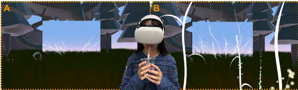
Figure 1: PlantSelf interaction. (A) The initial state where the user sees their plant avatar in a mirror within a calm VR environment. (B) After drinking water using the sensor-enabled straw, the virtual plant grows.
