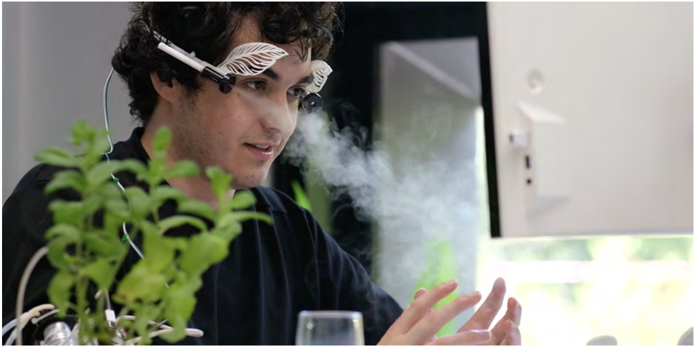
Figure 1: SymbioSip, a novel bidirectional hydration system designed to facilitate awareness of human-plant symbiosis. In this photograph, the system has detected that the linked plant needs water and so is supplying a mist to the wearer.
