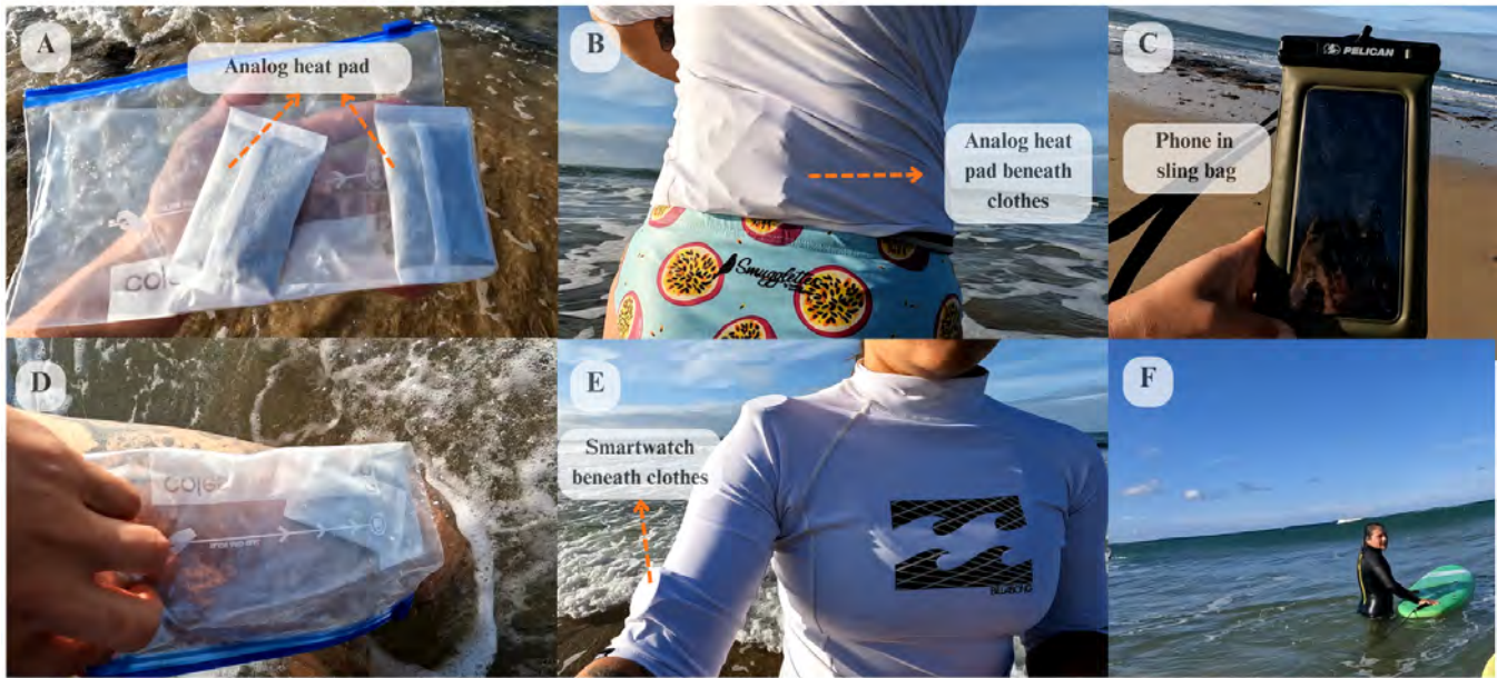
Figure 4: A) Analog heat pad in a plastic bag. B) Analog head pad placed on the back. C) Phone in a sling bag used to play pre-recorded sounds while surfing. D) Analog head pads placed on the leg. E) Samsung smartwatches placed on the arm are used as vibrotactile actuators. F) Exploring the sounds provided by the phone while surfing.
