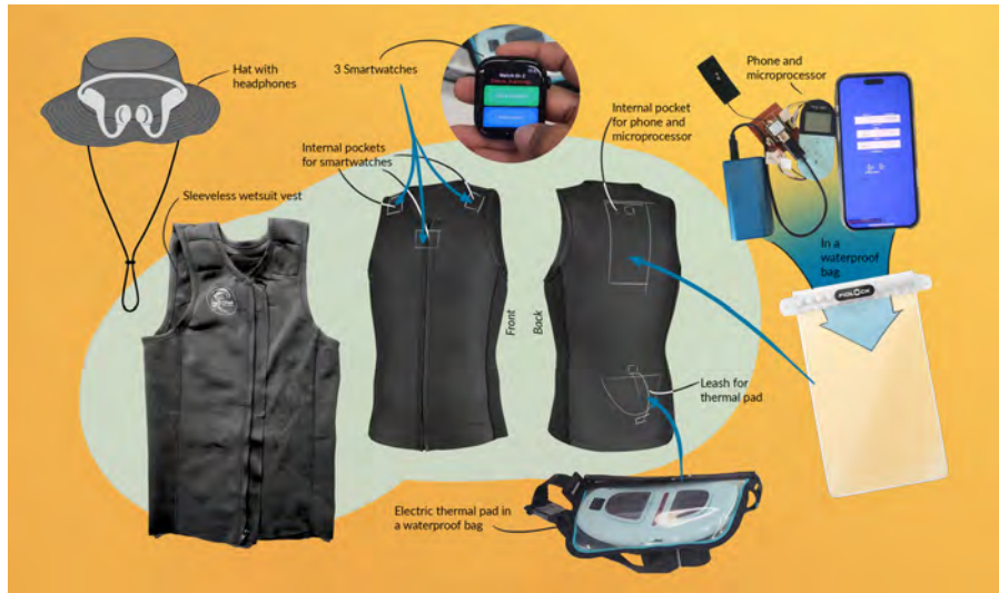
Figure 5: SurfSync component: a surfing vest with custom-made pockets embedded with a thermal pad and smartwatches controlled with a mobile phone app and a microcontroller, connected to bone conduction headphones embedded in a surfing hat.
