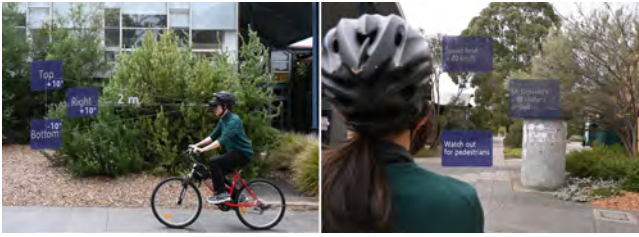
Figure 1: The experimental setup of user study 1 [9]. Left: An illustration of the notification placements. Top (elevation +10^\circ ), Right (azimuth +10^\circ ), and Bottom (elevation -10^\circ ). The placement is fixed at an optical distance of 2m from the user. Right: Participant's view of the bottom notification. Here, the bottom notification is displayed with higher brightness, while the top and right notifications are dimmer to indicate their relative placement.
