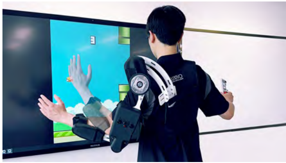
Figure 3: In SyncedWings, a player wears an exoskeleton on one arm and a controller on the other. If the AI predicts successful pipe avoidance, the exoskeleton mirrors the player’s actions, maintaining symmetry. Should a collision seem likely, it alters its movement to prevent it, requiring players to adapt their gestures accordingly.
