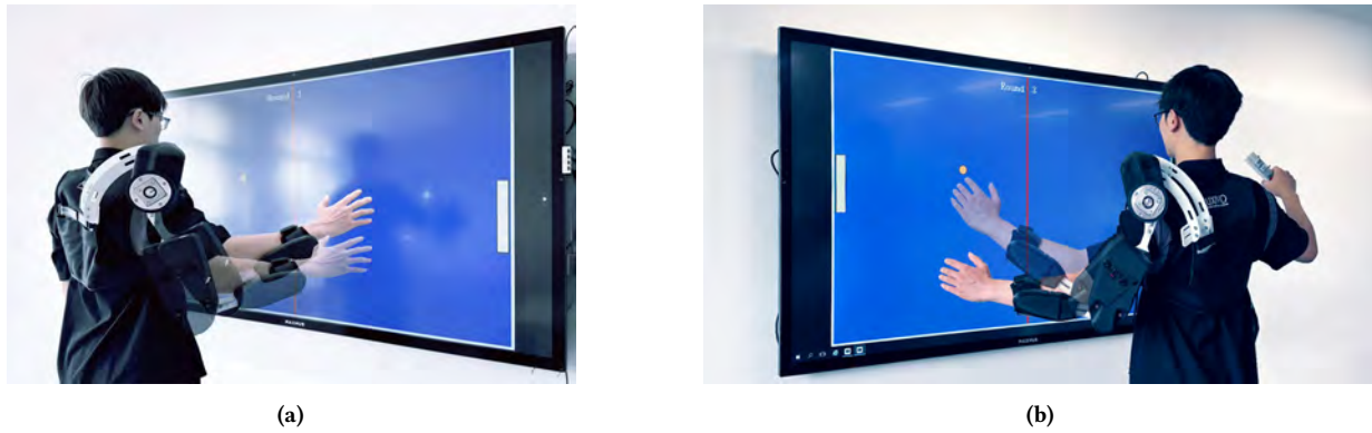
Figure 2: (a) In Proxy Pong, the player wears an exoskeleton on one arm. If a ball approaches the digital paddle of the human player side, the AI-powered exoskeleton actuates the player’s body to strike the ball. (b) In DualForce Pong, the AI-powered exoskeleton controls one digital paddle and the player swings their arm with the controller to manipulate another paddle.
