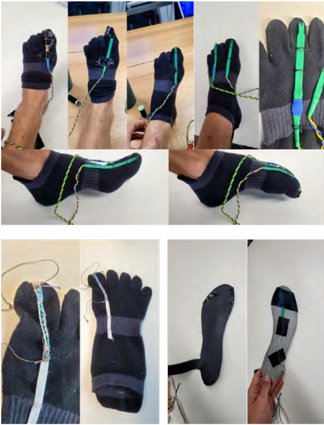
Figure 4: Explorations with flex sensors (left), stretch sensors on the toe (center) and pressure sensors on the insole (right)
