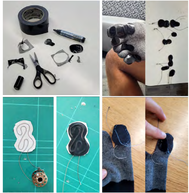
Figure 5: Crafting the prototype, determining the size of the sensors, creating the pressure sensors, sewing them on the sock
