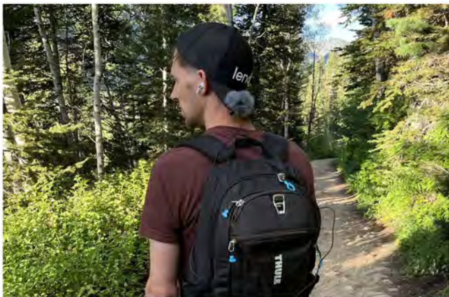
Figure 4. “Conversation Mute” manipulates engagement with other people on a hiking trail by playing nature sounds in earbuds to drown out loud conversations on the trail. This picture shows testing of a low-fidelity prototype on a hiking trail. The microphone clipped to the cap records audio which is transmitted over a wire to a laptop in the backpack.
