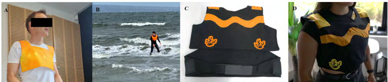
Figure 4: Wearable top prototyping A) The wearable top made in thermochromic fabric with colour-changing activation due to the vibration motors. B) A volunteer surfer testing the top. C) the wearable top is made with expanded fabric and thermochromic fabric in the shoulder, collarbone and waist areas. D) User wearing the wearable top with embedded electronics, with colour-changing activation due to head pads.
