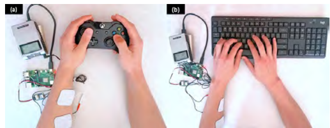
Figure 2: Wi-Fi Twinge usage scenarios: (a) Finger flexion affects operating a controller; (b) Finger flexion affects typing at work.
