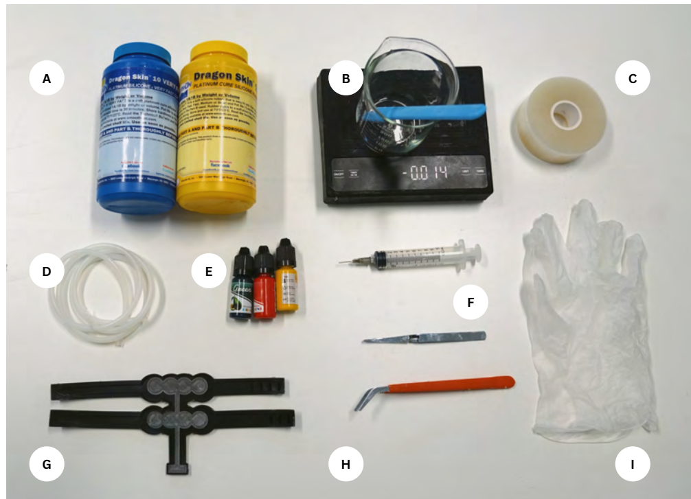
Figure 3: Fabrication kit for creating silicone-based bodily extensions. A) Liquid silicone; B) Weighing scale and a beaker for mixing silicone; C) Silicone tape for sealing the bodily extensions post fabrication; D) Silicone tube to connect the bodily extension to the pneumatic controller; E) Silicone dye; F) Piston for injecting water during fabrication; G) A 3D printed mold and PVA-based separator for the "Greetings" bodily extension; H) Tweezers to add the separator to the silicone layer; I) safety gloves
