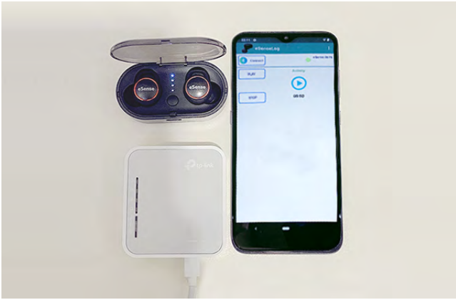
Figure 6: Each participant received a package containing the GustosonicSense system that consists of the earbuds, the smartphone with our customized application, and a router.
