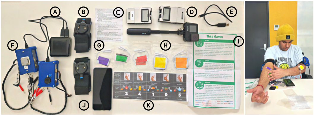
Fig. 3. (Left) shows the computational EMS system provided to the participant for the study. (A) cables and power bank, (B) two Velcro arm bands, (C) EMS safety instructions, (D) two EMS devices, (E) additional charging cable, (F) microcontroller devices, (G) colour-coded electrodes, (H) GoPro camera, (I) games description leaflet, (J) phone with a software application installed, and (K) instruction sheet showing hand-gestures and associated meanings for the games. (Right) shows a participant calibrating using instructions on (J) during the pre-study session.
