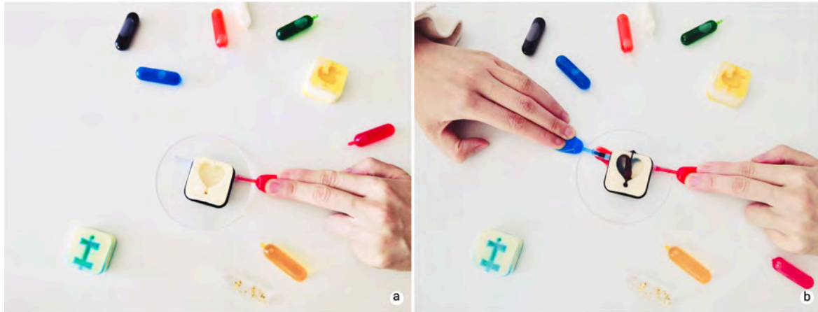
Figure 5: Eating a Logic Bonbon with an AND gate. a) No flavor outcome inside the logic Bonbon when only one flavor input is on; b) The flavors are mixed inside the Logic Bonbon when both inputs are on.
