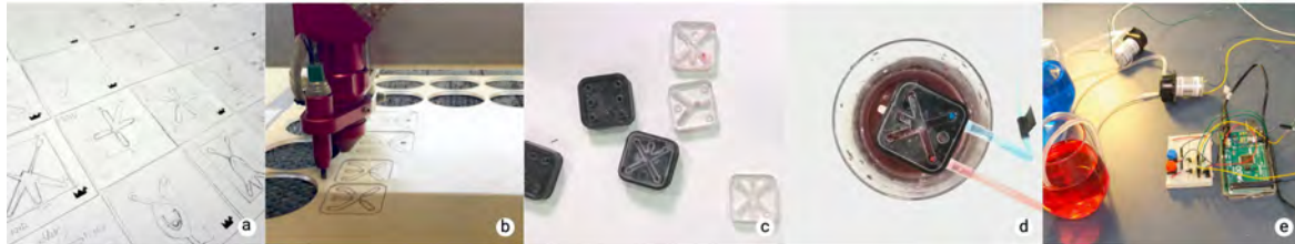
Figure 2: Prototyping the fluidic system. a) Design sketches of fluidic configurations; b-c) Fabrication of the fluidic devices; d-e) Testing the fluidic system.
