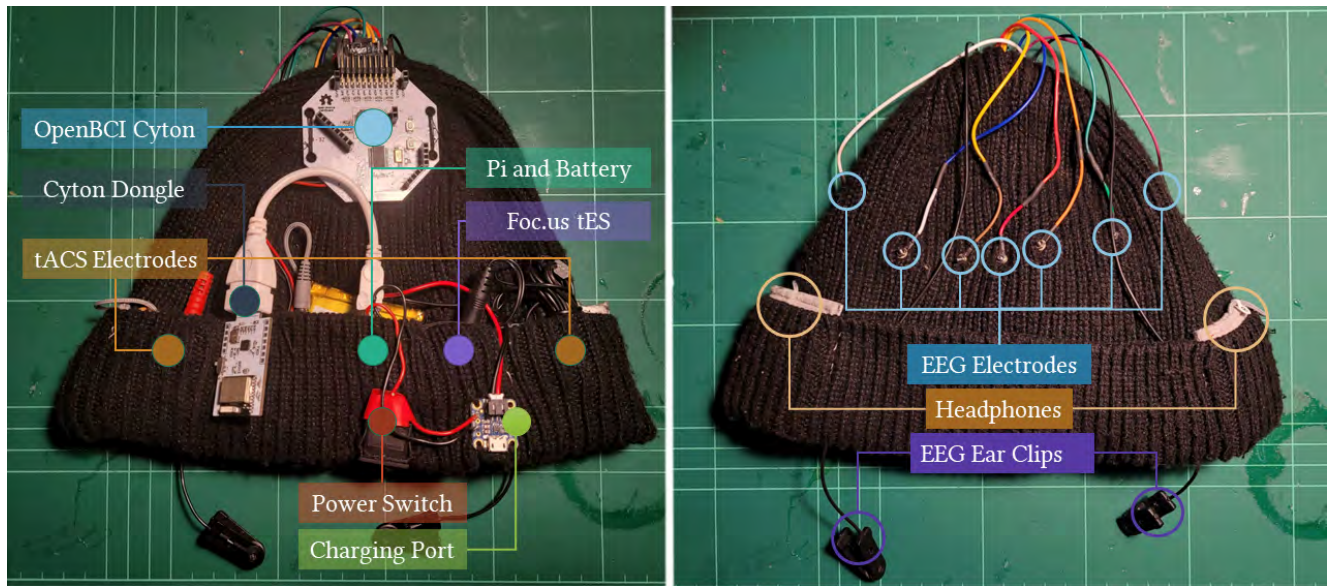
Figure 2: Dozer components. Left shows the front of Dozer with the outer layer removed, exposing the inner hardware. This includes the OpenBCI Cyton board for EEG data acquisition, a Cyton Bluetooth dongle to transmit EEG to the raspberry pi, a raspberry pi zero which is powered by a lipo battery, processes EEG data and initiates stimulation, a foc.us tES device that administers the tACS stimulation after receiving an initiation command from the raspberry pi, and a power port and switch to charge and power on/off the device. Right shows the back of Dozer with the outer layer removed, visible are the EEG electrode wires entering the beanie from the back, along with two headphones for administering pink noise stimulation after receiving an initialisation command from the raspberry pi, as well as ear clip electrodes that serve as ground and reference for the EEG. In both images, most of the hardware is tucked into the fold of the beanie.
