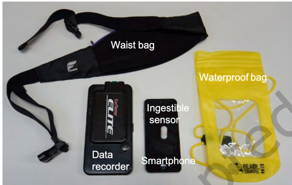
Fig. 4. The equipment we gave to players. The waist bag was used to contain the data recorder so that players could wear the recorder around their waist. The waterproof bag was for players to put the smartphone into when showering or swimming.
