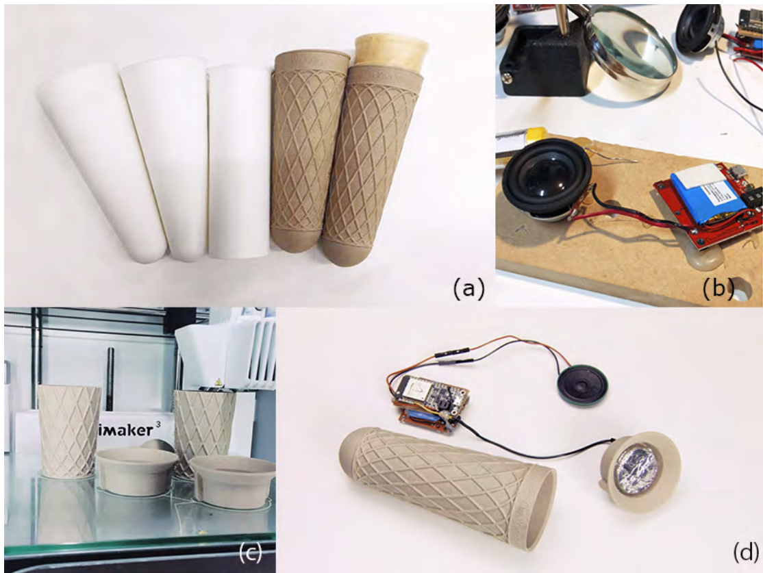
FIGURE 5.2: (a) The iterative 3D-printed cone; (b) a Bluetooth speaker board paired with a speaker; (c) a light wood filament for the 3D-printed cone; (d) the WeScream! configuration.
