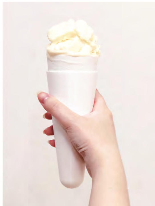
FIGURE 4.2: The 3D-printed cone contains a wireless microcontroller connected to removable food-safe aluminium foil that then makes contact with the ice cream.
