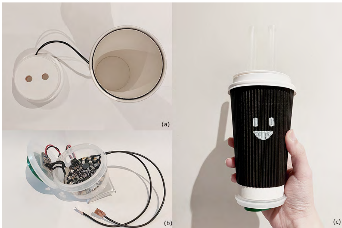
FIGURE 6.6: (a) A customised lid with two holes; (b) the electronics in the bottom container; (c) the Sonic Straws system with all components.
