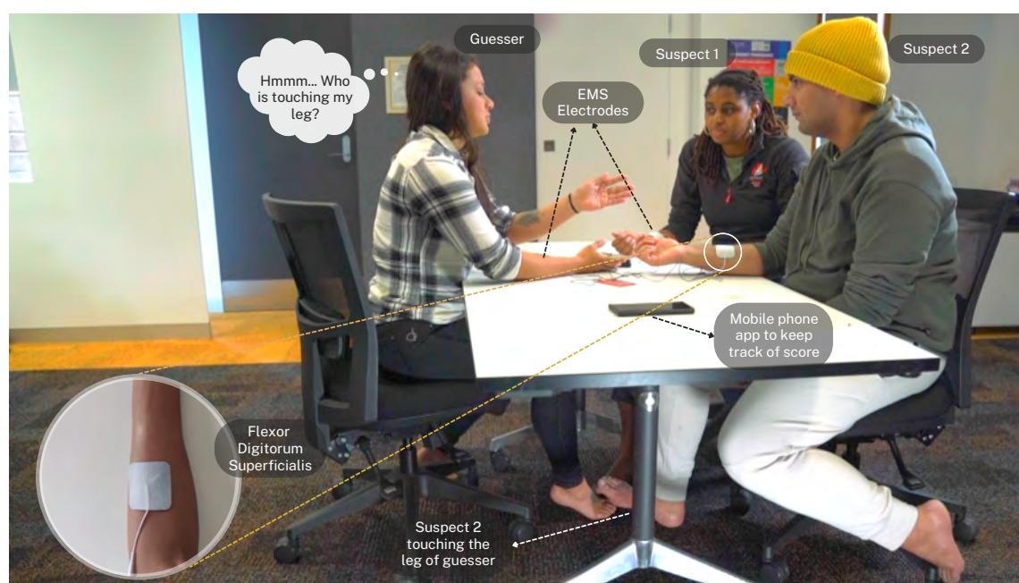
Fig. 1. Shows one guesser and two suspects on either side of the table. The guesser had the ground and each suspect had an active electrode from one EMS channel attached to their forearm. Here, suspect 2 is touching the guesser's foot, actuating the guesser's and their own hand. The guesser is pointing correctly towards suspect 2, winning this round.
