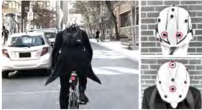
Figure 3. Ena in action (left). Data is streamed via electrodes O1 and O2 (top), with AFz as ground and CPz as reference (bottom).
