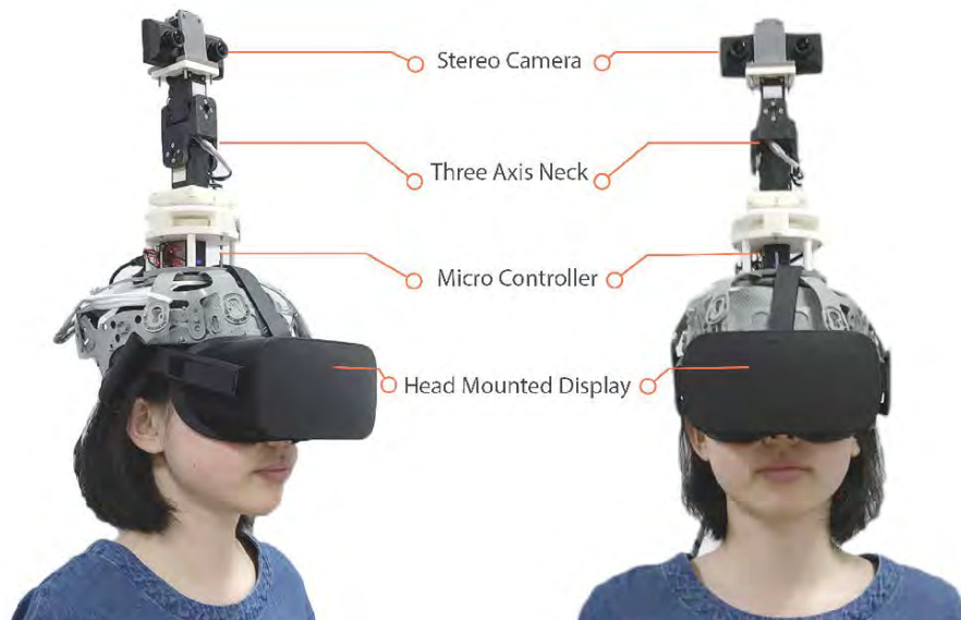
Fig. 3. This wearable robot augments the wearers neck by expanding their range of visual motion in space, thereby influencing their visuomotor processes. [12]
