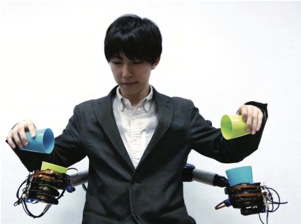
Fig. 2. MetaLimbs, a HInt system which extends the users body through two additional robotic arms. [10]
