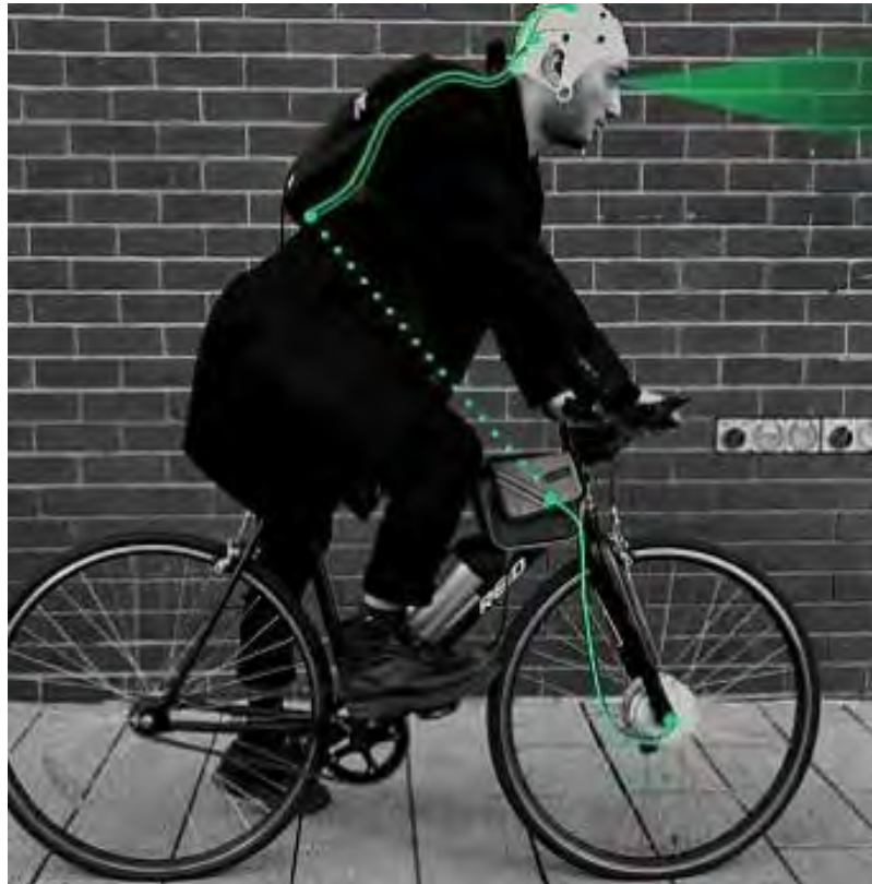
Fig. 1. Ena, an e-bike which integrates with the riders visual cortex through EEG, allowing the bike to detect sudden changes in the riders peripheral vision. [1]
