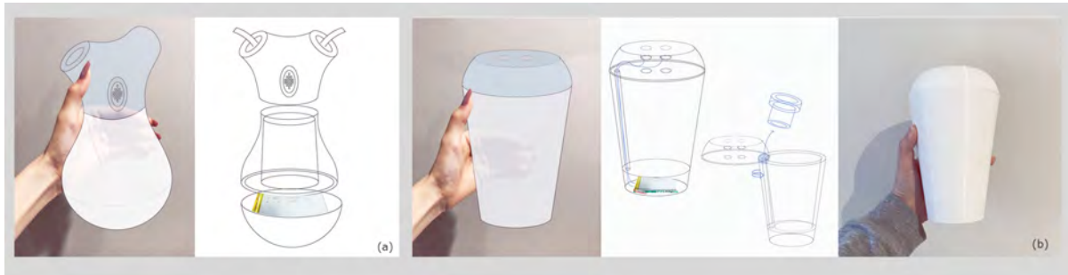
Fig. 4. (a) In the first design, a speaker and a microcontroller were placed into a lid structure; (b) in the second design, a replaceable cup was covered with a 3D-printed cover.
