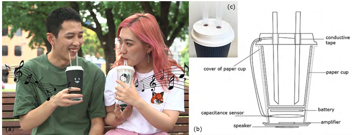
Fig. 1. (a) Sonic Straws is a beverage-based gustosonic system that supports the experience of playful personalized sounds via drinking beverages through straws; (b) Sonic Straws consists of a paper cup, a customized lid, and a holder; (c) the customized lid with two holes includes removable copper conductive tape for sensing via the straws.
