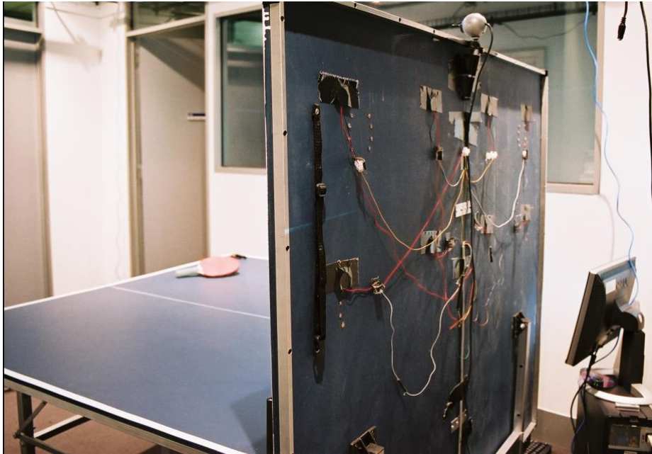
Fig. 4. Sensors attached to the back of the Table Tennis for Three system.
