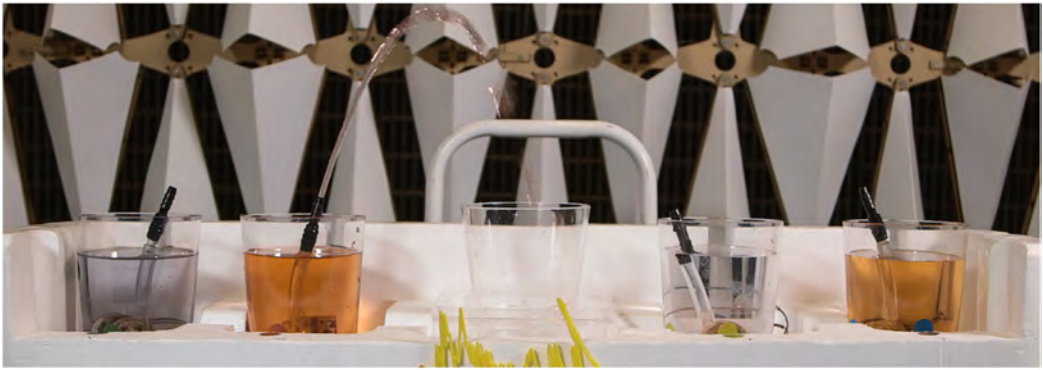
Fig. 2. TastyBeats is a fountain-based interactive system that creates a fluidic spectacle of mixing sport drinks based on heart rate data of physical activity.
