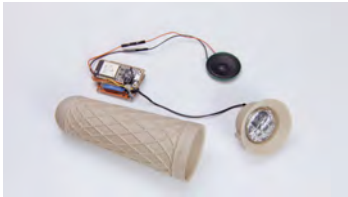
Figure 2: The 3D-printed cone contains a wireless microcontroller connected to removable food-safe aluminium foil that then makes contact with the ice cream.
