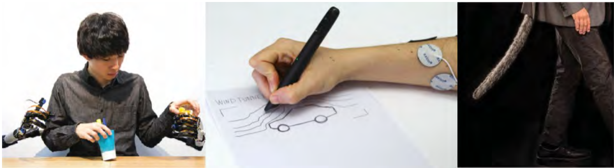
Figure 1. Exemplars of Human-Computer Integration: extending the body with additional robotic arms; [71] embedding computation into the body using electric muscle stimulation to manipulate handwriting [49]; and, a tail extension controlled by body movements [87].
