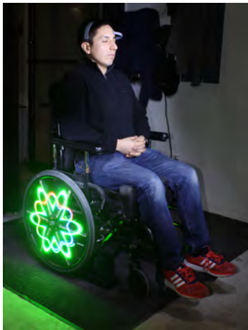
Figure 3: Self-driving wheelchair with “cyborg-motor-memory” for an electric motor [30]. A linear array of light sources on each spoke assists with biofeedback-based motor memory training.
