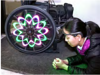
Figure 2: Mind over Motor: Testing a self-driving wheelchair with brain-computer interface (BCI) and biofeedback [30].
