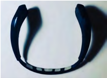
Figure 3: We use MUSE EEG headsets to read the electrical activity that is occurring inside the brain.
