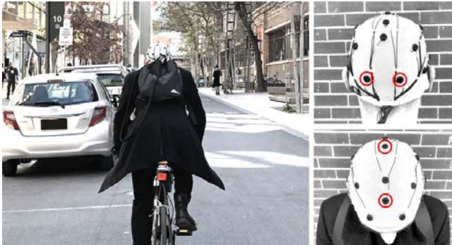
Figure 3. Ena in action (Left). Data is streamed via electrodes O1 and O2 (top), with AFz as ground & CPz as reference (bottom).
