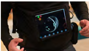
Figure 3: InsideOut uses a wearable display showing the user real-time video of their GI tract.
