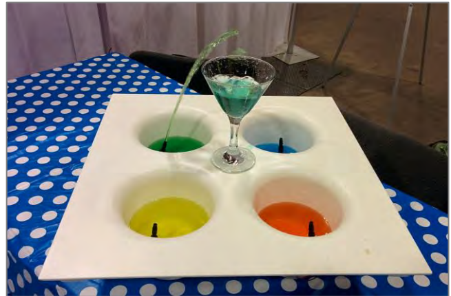
Figure 5: TastyBeats' water pumps shoot the drink's liquid into the central glass
