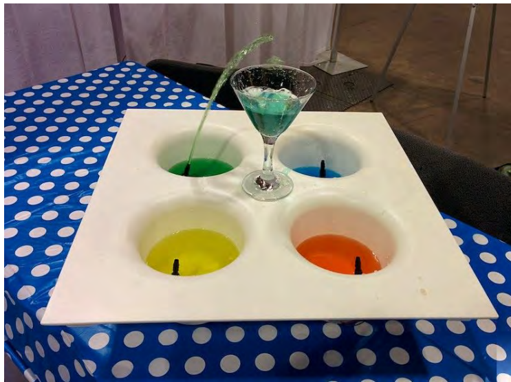
Figure 25: The TastyBeats © (Khot et al., 2015b) creates visual fluidic spectacle of someone's physical activity.
