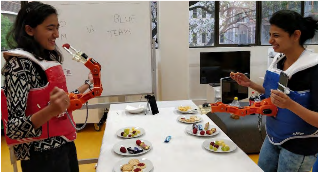
Figure 20: Arm-a-Dine © (Mehta et al., 2018) support playful mealtime conversations through on-body robotic arms.
