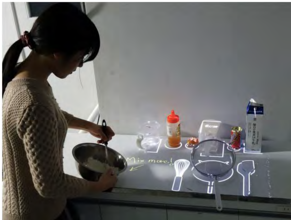
Figure 6: In the Shadow Cooking system (Sumriddetchkajorn, 2013), cooking instructions are projected onto the kitchen counter and they move forward according to the user's progress.
