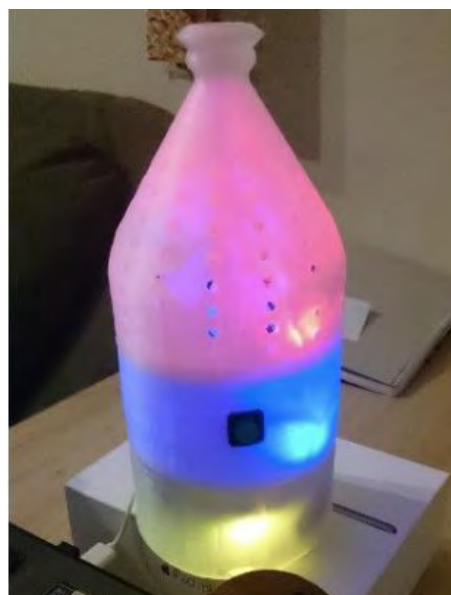
Figure 8: The Talking Bottle system (Sumriddetchkajorn, 2013) communicates the availability of voice messages or that someone is cooking in the remote kitchen through LEDs.
