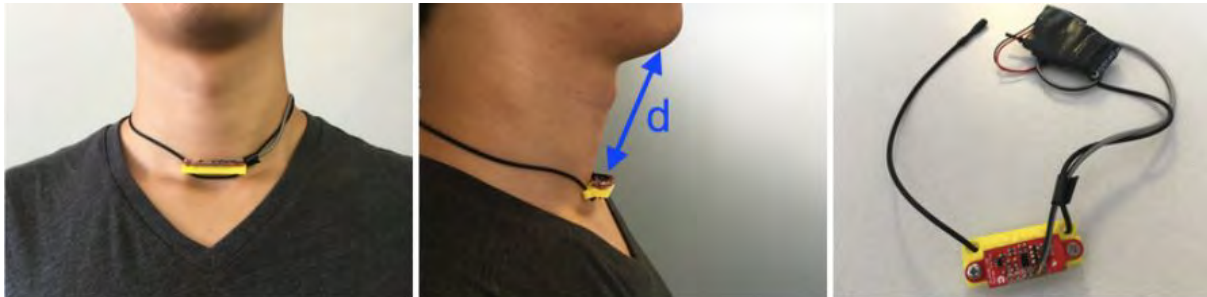
Figure 16: Chun and colleagues used proximity sensors to detect eating episodes © (Chun et al., 2018) .
