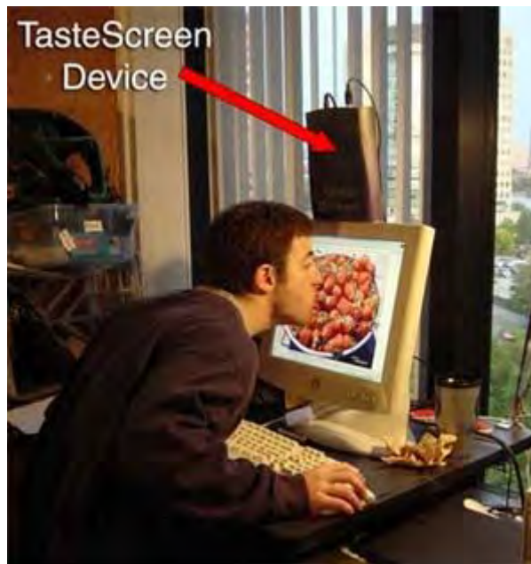
Figure 25: The TasteScreen © (Maynes-Aminzade, 2005) allows users to virtually taste different food items by licking their photographs displayed on an LCD screen.
