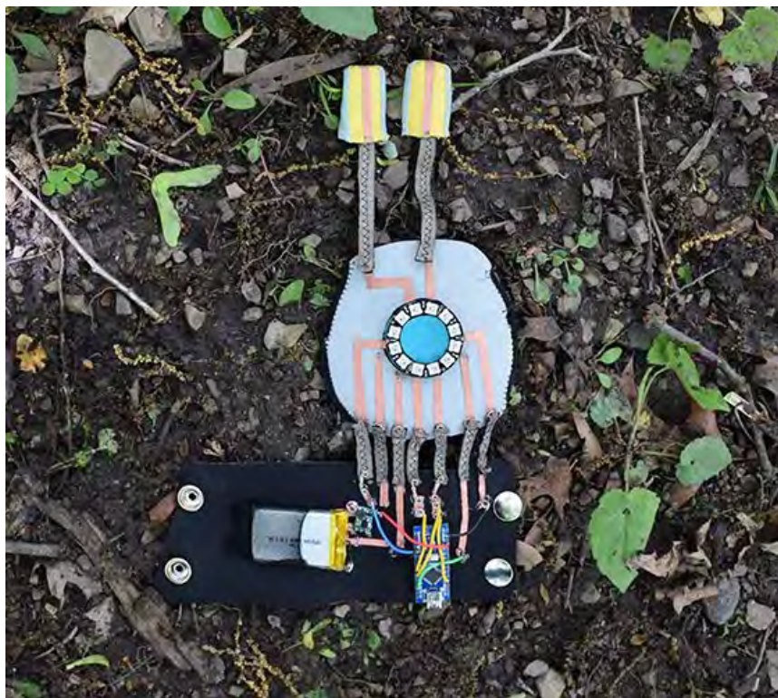
Figure 4: Hand-Substrate Interface (Sumriddetchkajorn, 2013) offers a direct engagement with the agricultural environment, wherein the wearer physically inserts their hand in the soil to obtain the soil moisture reading.
