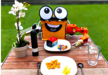
Figure 1: FoBo is a speculative design prototype for a mischievous robotic dining companion that acts and behaves like a human co-diner.
