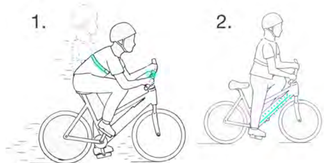
Figure 1. Ava senses the rider’s posture to activate: 1. the eBike’s engine acceleration according to the rider’s torso angle. 2. when going slow (resuming cycling) activating LED safety hazard.
