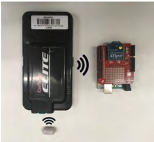
**Figure 4:** The Cortemp sensor transmits a signal to the Elite receiver every ten seconds. The Elite receiver then transmits the data to the Arduino.
