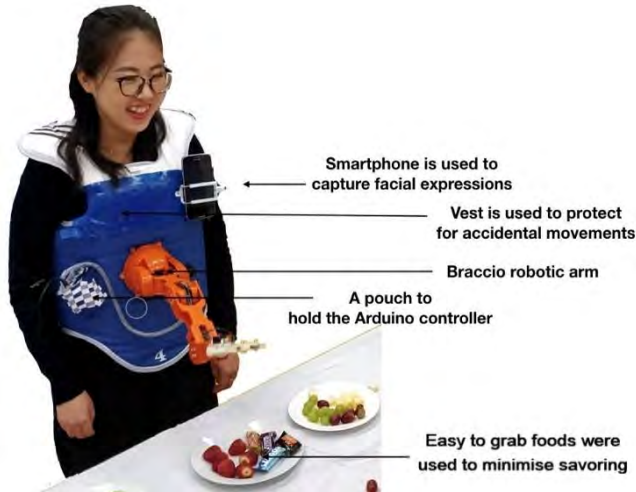
Figure 2. Arm-A-Dine features an on-body robotic arm (supporting the feeding action from plate to mouth) and an attached smartphone to capture facial expression of the eating partner.
