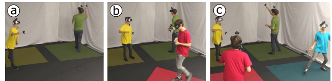
Figure 7: (a) VirtualSpace handles configurations with fewer users. (b) If free space is available, apps can perform different maneuvers at the same time, until (c) all space is allocated, then maneuvers need syncing.
