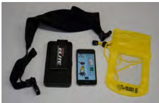
Figure 2: The players need to wear a waist bag containing the receiver. An iPhone is used to play the game. We also prepare a water-proof bag for the player in case they swim or shower during the gameplay. The pill is placed on top of the iPhone for size comparison.
