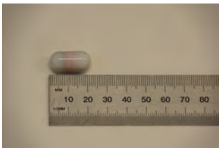
Figure 3: The Cortemp sensor is approximately 22mm in length.
