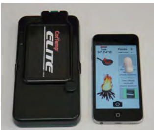
Figure 4: The device on the left is the receiver for the pill data. It passes the data on to the phone via bluetooth. The screen of the phone shows the interface of the game.
