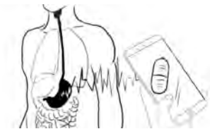
Figure 1: The ingestible sensor continuously captures the user’s body data and transmits it to a smartphone wirelessly.
