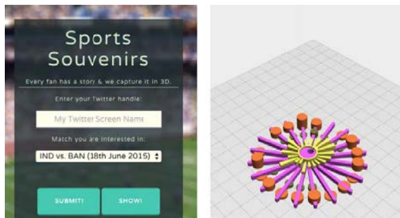
Figure 5: Screenshot of the system: a) Users enter their twitter handle and then select a match from the Cricket series. b) A 3D model of Fantibles is then created based upon the sports data and users’ own tweets during the match
