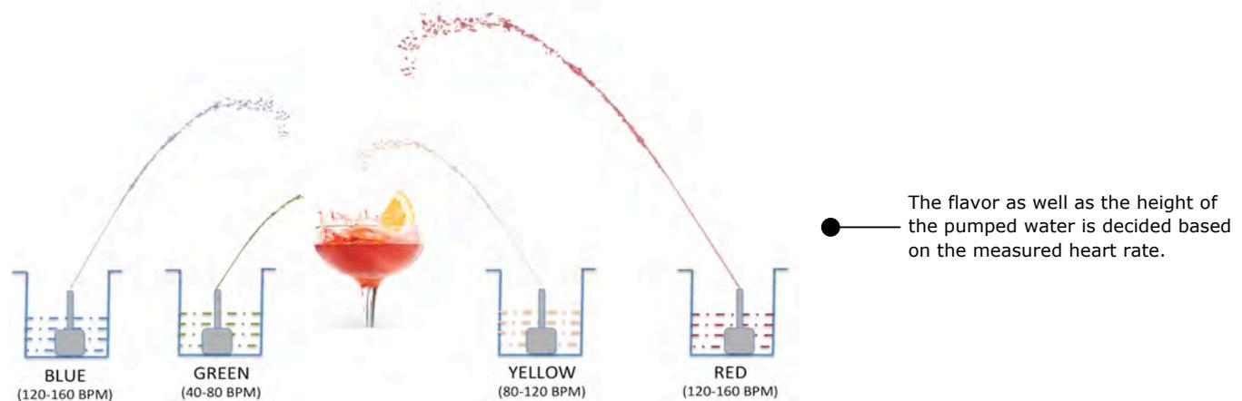
**Figure 3.** In TastyBeats, user creates a mocktail drink by mixing different flavors together, using his heart rate as control parameter.
