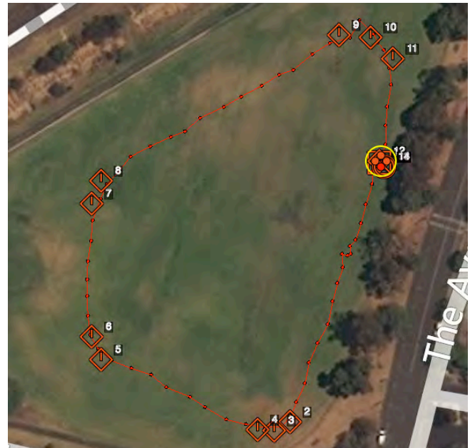
Figure 3. The waypoints and quadcopter flight path for a single jogging lap.
