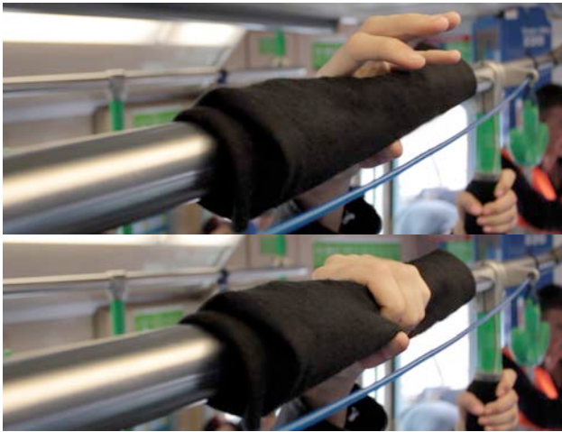
Figure 4. Cart-Load-O-Fun on a tram. The sensors attached to the bars are squeezed and released by a passenger to play the game.
