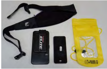
Figure 3: Hardware needed for the game: Mobile phone, the pill (located on top of the mobile phone), the receiver for the pill, a bag to carry the receiver and a waterproof bag for water based activities, e.g. showering (yellow bag).
