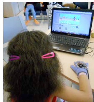
Fig. 6. The play characters are put on top of this augmented glove to control the game
