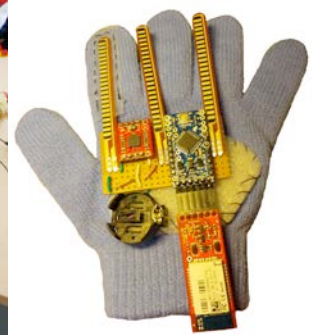
Fig. 6. The play characters are put on top of this augmented glove to control the game
