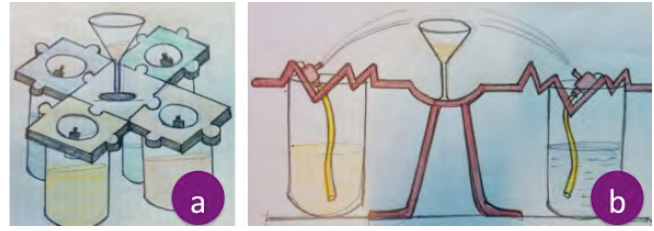
Figure 3: Other design options for TastyBeats were discussed but not considered due to a) less interaction possibility with equidistant pumps, b) self-priming issue with the pumps.
