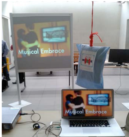
Figure 1. Musical Embrace setup: the laptop is for our analysis; players interact with the pillow-like controller with the option of watching the large screen.
